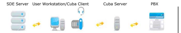
The PBX component above may be hardware or a software based server. The software server will ultimately communicate with telephone hardware. For example, Cuba Server connects directly via a network connection to an Avaya IP Office but via a CCT Server to a Nortel Meridian system. The common part is a 3<sup>rd</sup> party TAPI driver. This component is generally installed on the same machine which hosts Cuba Server.
