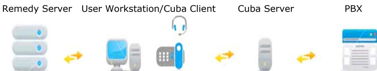
The Remedy Server is shown above for clarity. Note that interaction between Cuba and Remedy is via the client. Cuba client communicates with Remedy client to search or submit data to a Remedy database. Cuba client can be configured to communicate with Remedy thick (Windows User) or thin (web based) clients.
